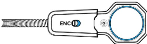
When the switch is pushed away from the ENC position, the ENC function is disabled, and the microphone boom indicator turns off.
