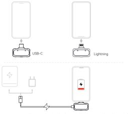
\*Supports charging the device via RX when smartphone battery is low.
