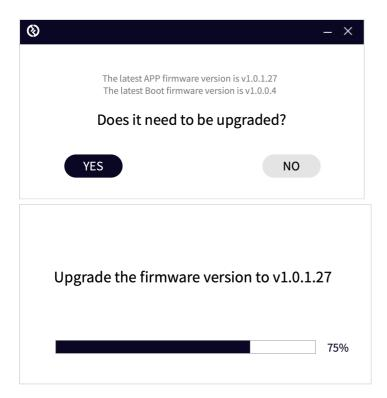
Note: Don't unplug the USB cable until it upgrades successfully. (The box indicator light will be off for about 5-10s when upgrading)
