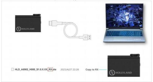
4. After copying successfully, unplug the USB cable and it will do the upgrade automatically.
