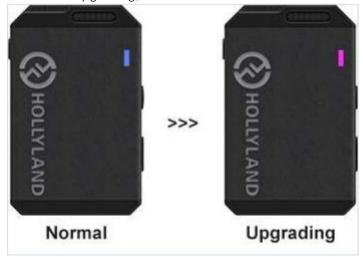
4. After upgrading successfully it will reboot, you can check the firmware on the receiver.
