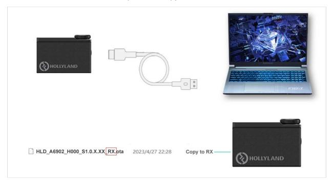
4. After copying successfully, unplug the USB cable and it will do the upgrade automatically.
