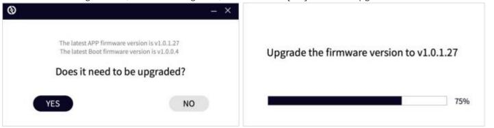
Note: Don't unplug the USB cable until it upgrades successfully. (The box indicator light will be off for about 5-10s when upgrading)
