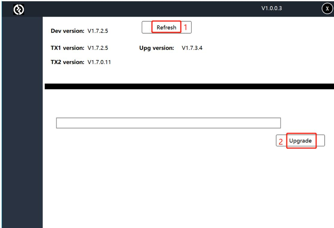
Then the RX will upgrade the TX in turns wirelessly. (The TX will turn purple when upgrading)
