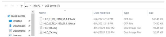
3. Connect the USB disk to Mars 400S Pro via type-C port, it will recognize the USB disk automatically and start to updating
