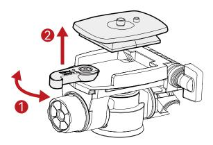
2. Attach the quick-release plate to the camera's 1/4" threaded hole, then snap the plate into the tripod mount.
