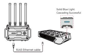
Insert the beltpack vertically into the cascaded charging base. After approximately 3 seconds, the beltpack will automatically pair with the current cascaded system.
